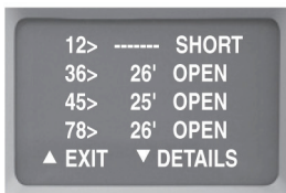
Figure C-3. Bad cable: near-end short.
